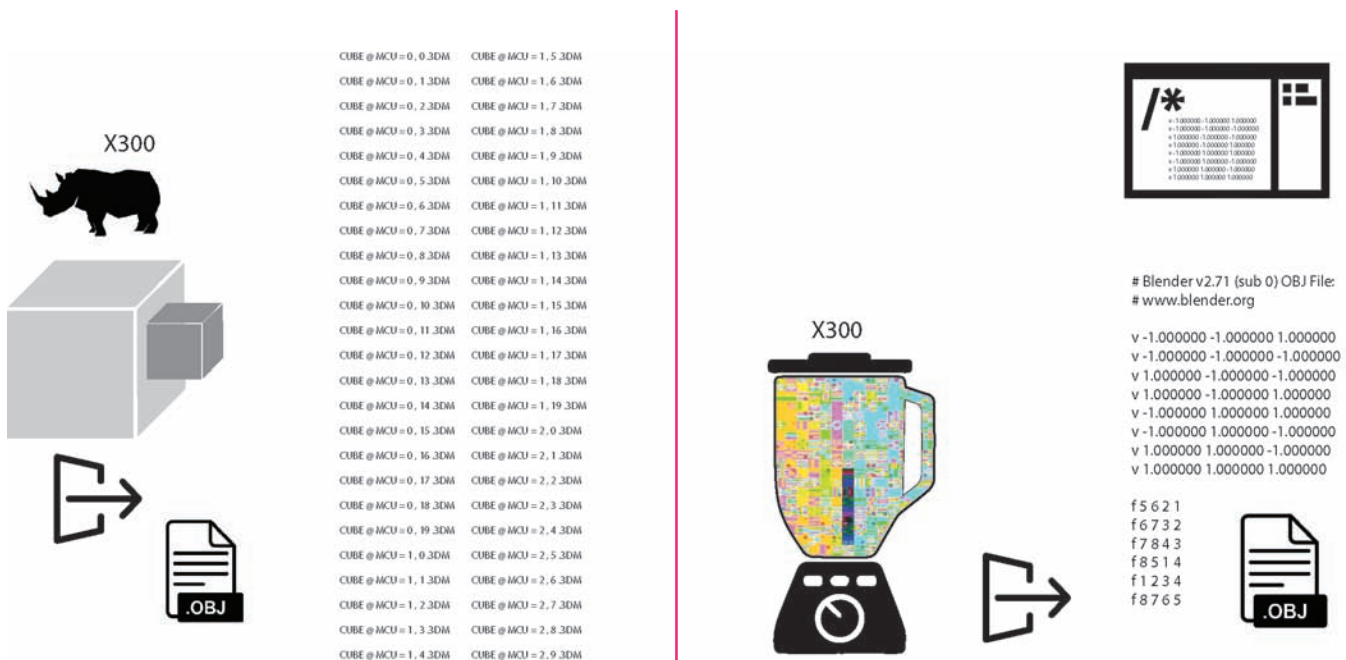
Figure 6.61 Diagram explaining the design progress shifting from Rhino to .obj export format imported into Blender for vertices's shifts, again exported as .obj
